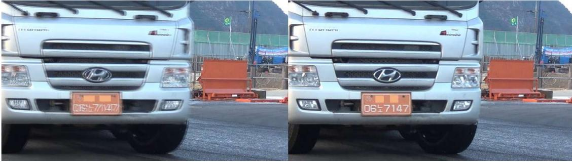
Figure 2. Effects of video deinterlacing (Left: before deinterlacing, Right: after deinterlacing).
