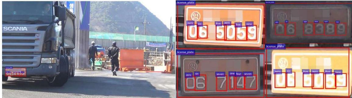
Figure 5. Examples of the license plate detection results (Left: a detection result in a video frame, Right: detection results enlarged at license plates).
