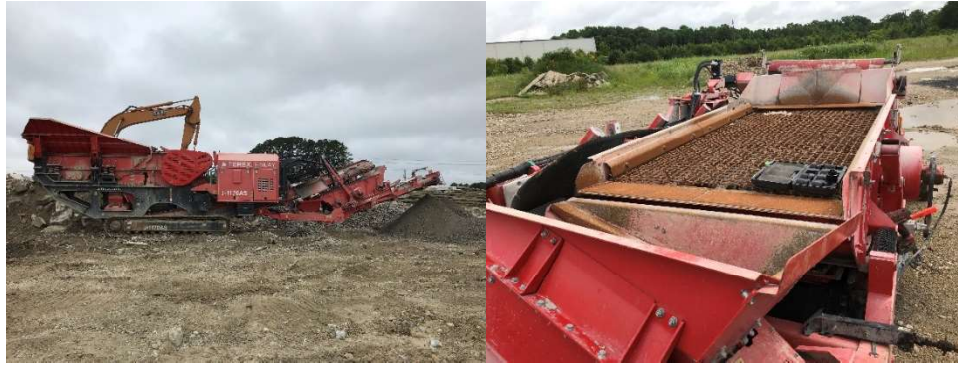
Figure 5: Concrete slabs removed - Terex Finlay J-1170 compact and tracked jaw crusher for RCA processing; (left); 1.5-inch screener for RCA used in the concrete (right).
