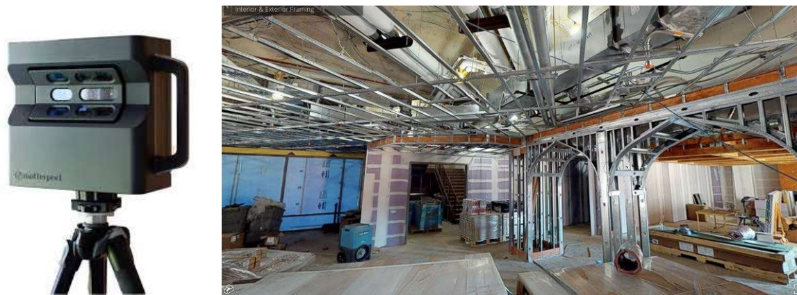
Figure 1: 3D scanner used and a screen capture of the virtual environment
