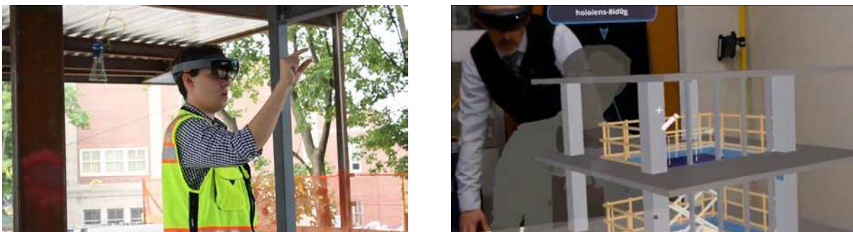
Figure 1: Use of MS HoloLens for Hazards Identification and Safety Planning. (images courtesy HITT Contracting)
