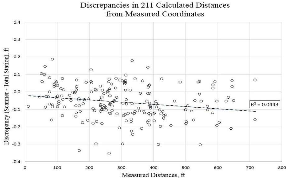
Figure 3: Discrepancies in Measured Distances from Chosen Center Points (T9, N1, N2, N3, S4 and S6)
