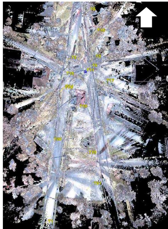
(b) Bird-Eye View of Full Point-Cloud Model Showing the Location of Target Points
