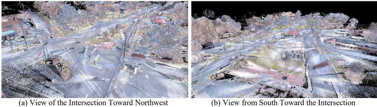
Figure 2: Final 3D Point-Cloud Model of the Selected City Intersection (with 3 converging streets and 2 railroads)
