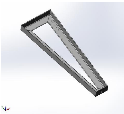
Figure 3(a): Steel base.
