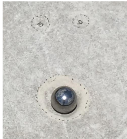
Figure 3: Passed dent from 3 in. steel ball test compared to dents from a 1 ¾ in. steel ball tests
