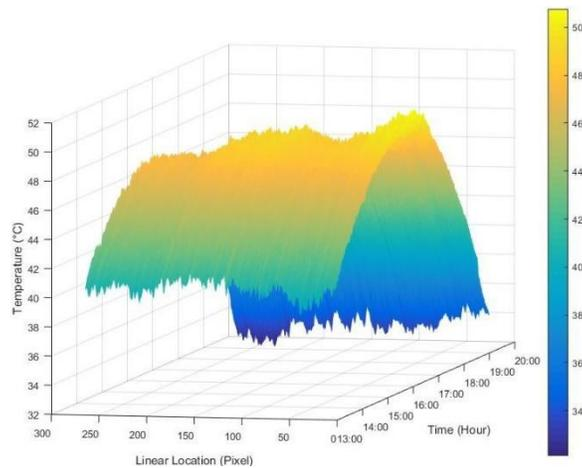
Fig.5 Variation of temperature with location and time on Line 3 (south wall vertical line)
