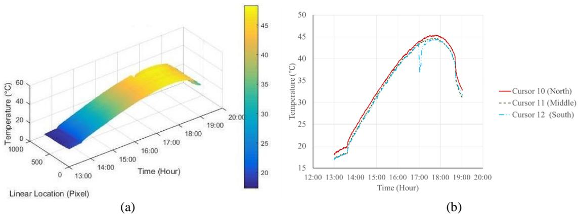
Fig.7 Variation of temperature on Line 5 (west wall lower horizontal line) with location and time (a) 3D view (b) temperature profile of cursor 10, 11, and 12 on Line 5
