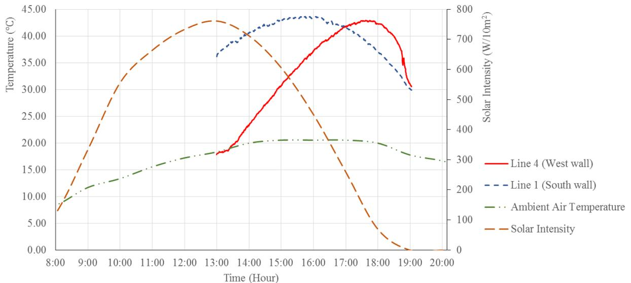
Fig.9 Timing of Different Peak Temperatures and Peak Solar Intensity
