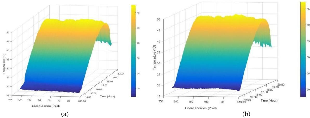
Fig.8 Variation of temperature with vertical location and time (a) Line 6 (west wall upper vertical line) (b) Line 7 (west wall lower vertical line)
