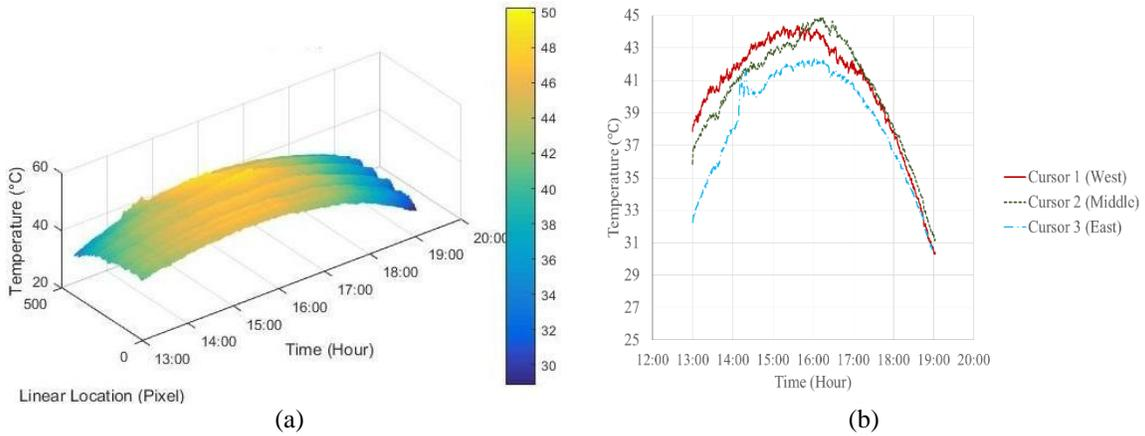
Fig.3 Variation of temperature on Line 1 (south wall upper horizontal line) with location and time (a) 3D view (b) temperature profile of cursor 1, 2, and 3 on Line 1
