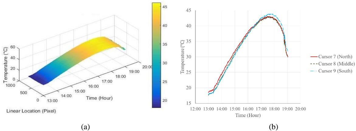
Fig.6 Variation of temperature on Line 4 (west wall upper horizontal line) with location and time (a) 3D view (b) temperature profile of cursor 7, 8, and 9 on Line 4
