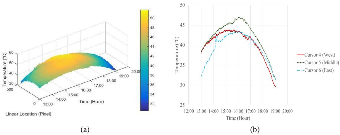
Fig.4 Variation of temperature on Line 2 (south wall lower horizontal line) with location and time (a) 3D view (b) temperature profile of cursor 4, 5, and 6 on Line 2
