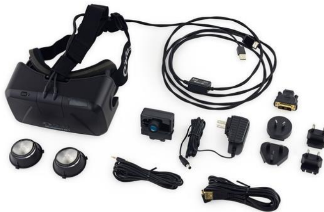
Figure 2: Components of Oculus Rift DK2. (Source: https://www.oculus.com )
