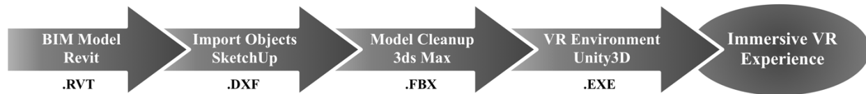
Figure 5: Modeling workflow for developing a VR environment for safety training.
