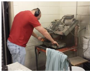
Cutting Asphalt Sample
