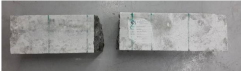
Figure 5: Beam flexural failure
