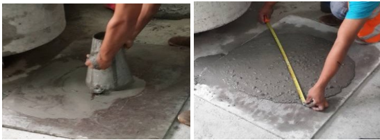
Figure 1: Slump flow test.
