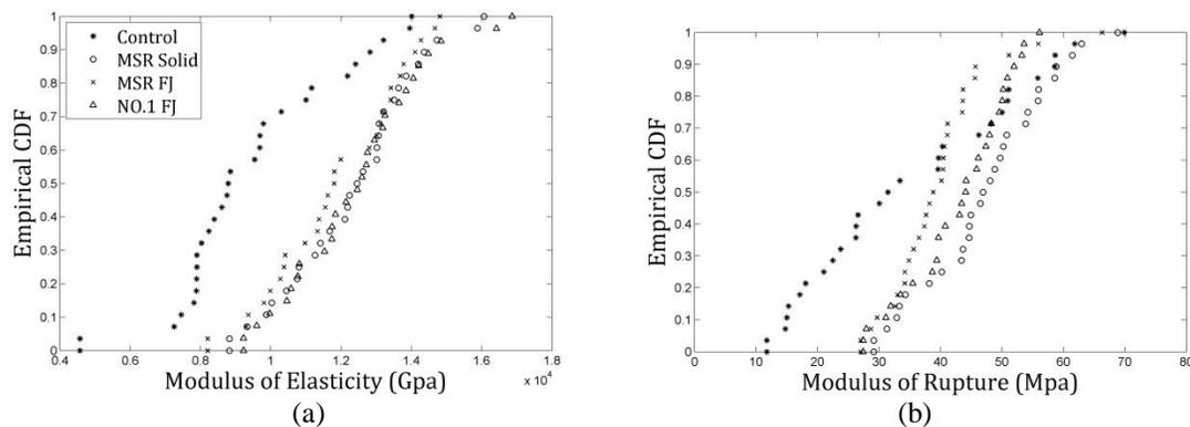
Figure 6: Cumulative Distribution Function: (a) Modulus of Elasticity; (b) Modulus of Rupture
