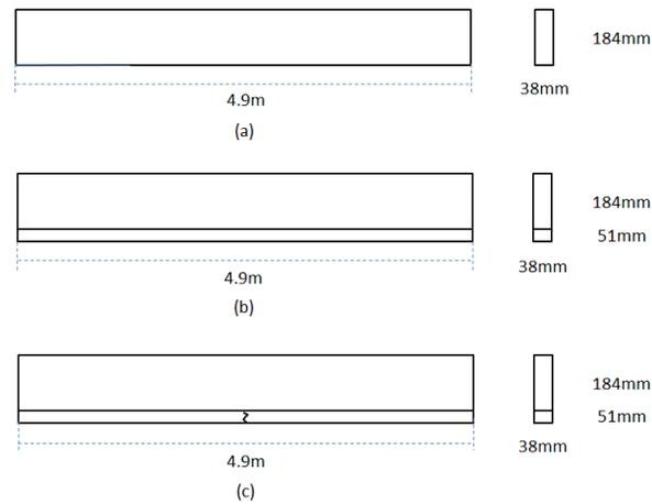
*Figure 2:* Dimensions of Test Lumber: (a) Control Chord; (b) TCL with Whole Piece Reinforcement; (c) TCL with Finger Joint Reinforcement
