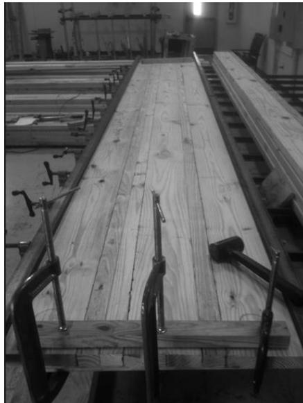
*Figure 3:* Photograph of the clamping system for manufacture of TCL specimens. In the clamps are three individual TCL specimens.
