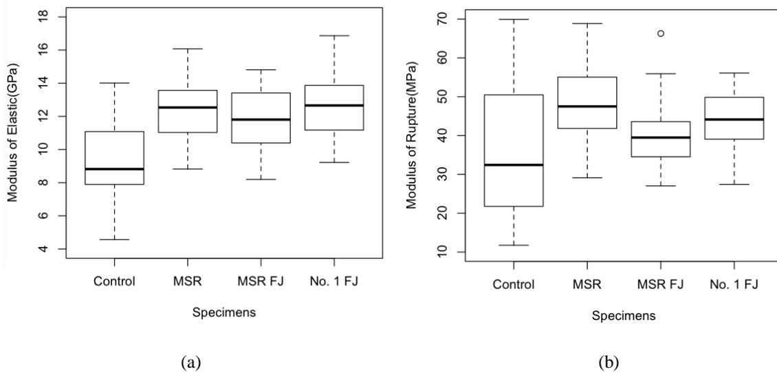
Figure 5: Boxplots: (a) Modulus of Elasticity; (b) Modulus of Rupture
