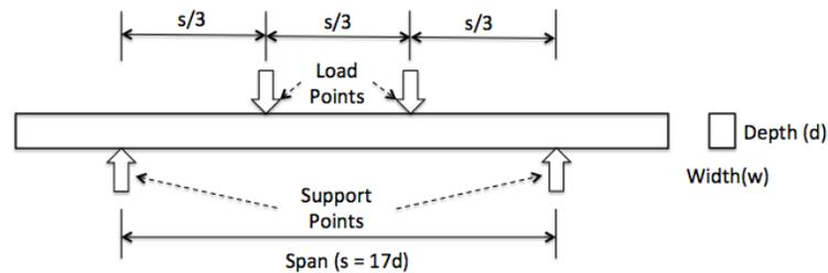
Figure 4: Third-point Loading Test Configuration for four-point bending
