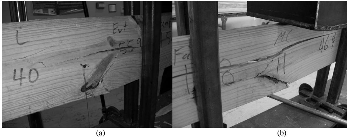
*Figure 1:* Typical failure mode of 2x10 lumber: (a) Failure above published design value; (b) Failure below design value.
