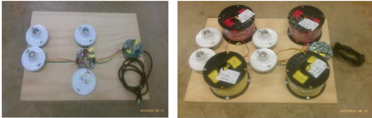
Figure 7: Photo of Completed Circuits Simulating Parking Lot Lighting Installations
