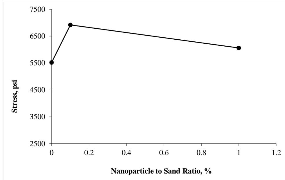
**Figure 5:** Effect of Nanoparticle on Strength
