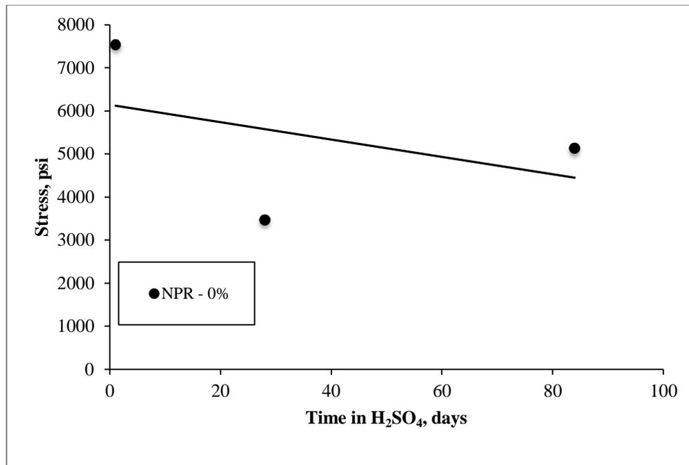
**Figure 6:** Effect of Sulfuric Acid Exposure on NPBC [NPR 0%]
