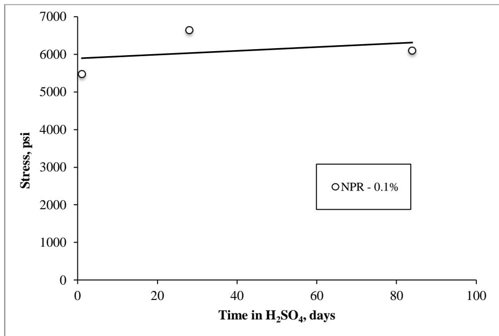
**Figure 7:** Effect of Sulfuric Acid Exposure on NPBC [NPR 0.1%]
