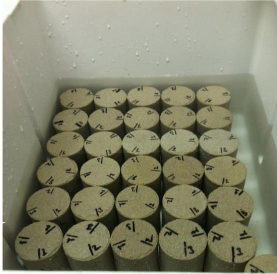
**Figure 3:** View of NPBC specimens immersed in 20% sulfuric acid solution
