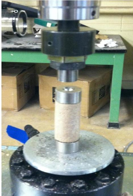
**Figure 2:** Hydraulic MTS System Used for Compression Testing
