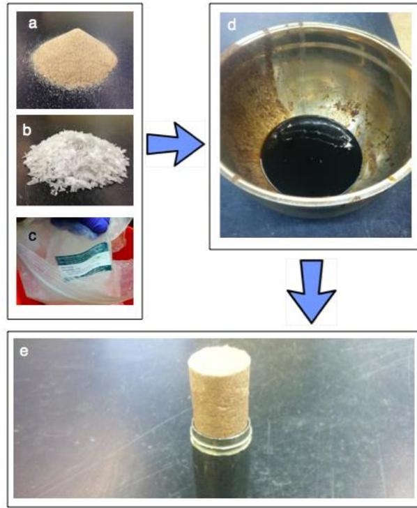
**Figure 1:** Sample Preparation of NPBC
