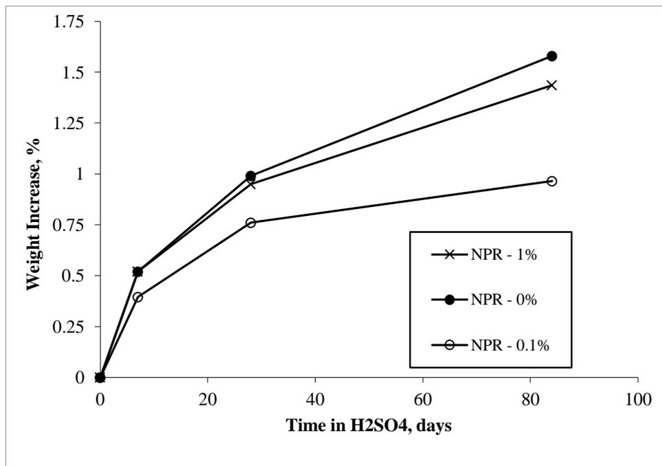
**Figure 4:** Effect of Acid Immersion on Weight Changes of NPBC
