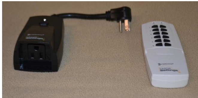
Figure 1: Retrofit WHS Disconnecter and Remote Control
