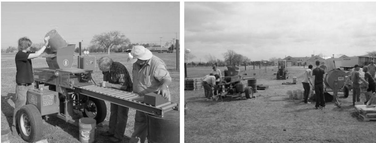
Figure 1: Left – CEB Block Machine Producing Blocks, Right – CEB Production Site
