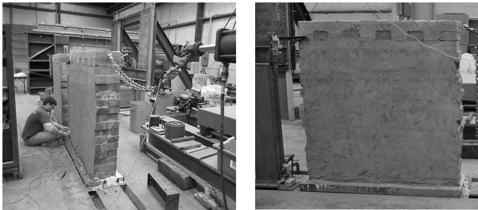
Figure 4: Setting up test walls to determine in-plane shear strength of CEB wall assemblies
