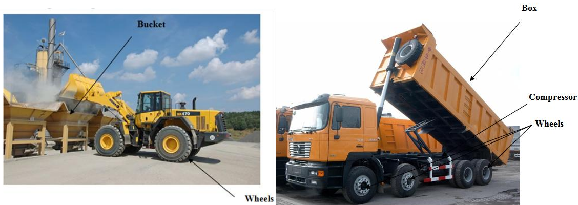
Figure 1: Dust Generation Sources in Typical Loaders and Dump Trucks
