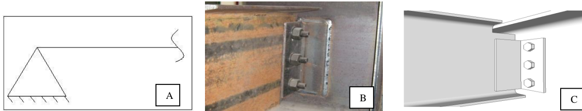
Figure 5: Complementary communication techniques to illustrate the fundamental principles of a pin connection to CM students: A) a line diagram is used to represent a pin connection in calculations and analysis B) an instructional steel sculpture is available to demonstrate the connection materially C) a rotatable computer model makes the connection easily viewable in 3D.
