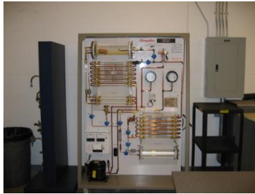
Figure 6: An equipment trainer with a glass evaporator and condenser
