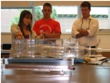
Figure 10: Students instruct students on static, velocity and total pressure with a model air handler
