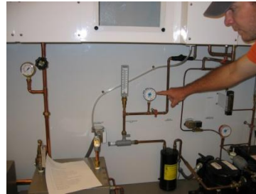
Figure 7: An equipment trainer using an instrumented 0.5 ton refrigeration unit
