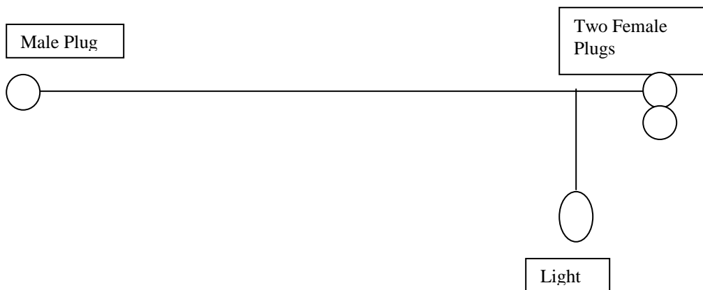
Figure 4 – Single Light Temporary Light
