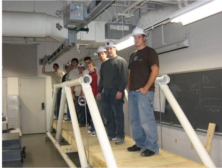
Figure 1. Completed PVC Bridge
