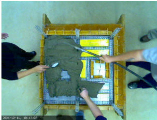
Figure 5: Placing the Second Floor
